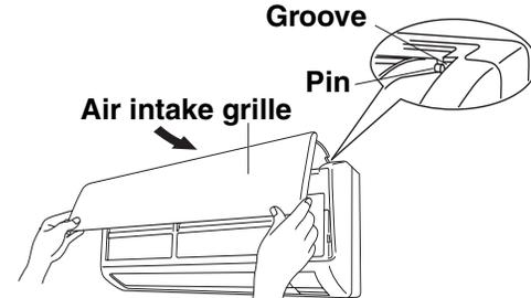
3. Press in the bottom right and left corners of the air intake grille to attach the indoor unit.
