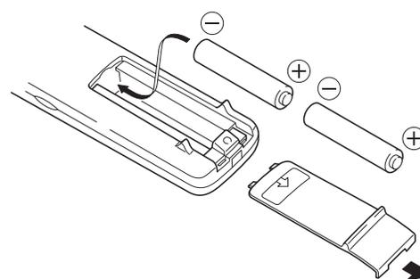
1. Slide the cover in the direction indicated by the arrow and remove it.
