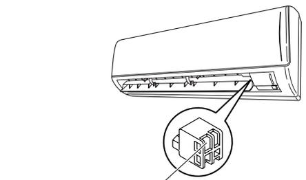
**Negative ion generator (metal electrodes inside plastic case)**
